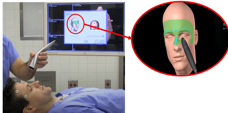
Figure 2: A surgeon performing patient-image registration by infrared scanning a patients facial surface. The scanned surface is then superimposed onto preoperative MRI images, as seen on the monitor.
