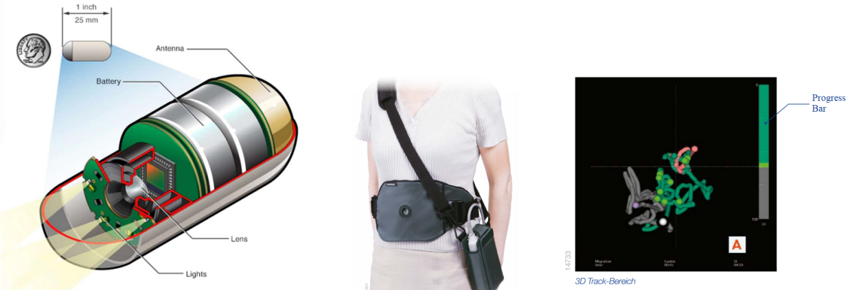
(a) The size and components of an ingestible endoscopy capsule
