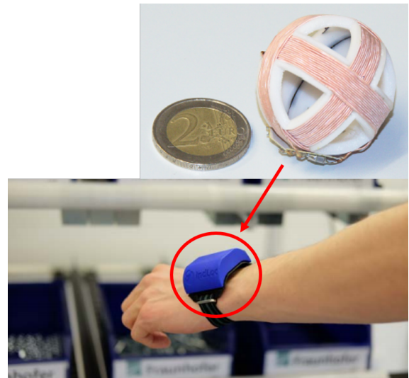
(b) The wearable is attached to the wrist and can be localized in real-time in 3D space
